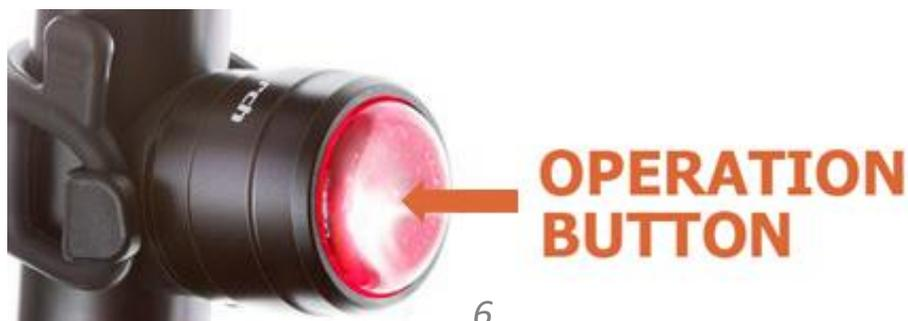
**Operation Modes:** The initial **two short presses** (or *single press for earlier models*) of the power button will turn on the light on High mode. Each additional short press of the button switches the light from one mode to the next, in the following order: (1) *High*; (2) *Slow flashing*; (3) *Quick flashing*; (4) *Pulse*; (5) *OFF*. Press & Hold of the power button will shut down the Tail Bolt.
